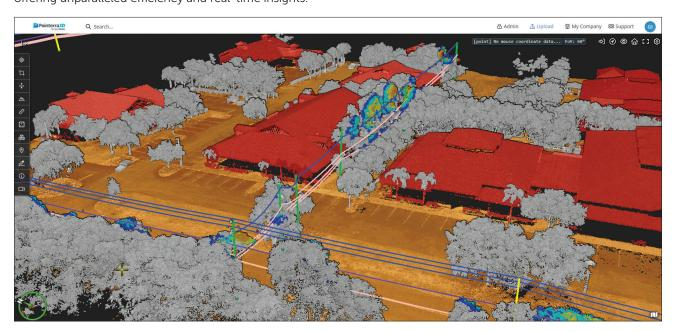
Addressing the need for speed in reacting to risk identification and mitigation, high-resolution LAS format point clouds from Network Surveyor are directly ingested into the Pointerra3D digital twin platform and support immediate vegetation encroachment analysis within mere hours of flight. Image courtesy Pointerra3D
