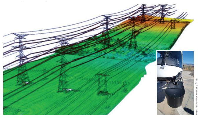
High-resolution lidar point clouds of utility assets deliver a 3D representation of infrastructure and surrounding objects to enable the fast identification of risks to assets, and public safety. Network Surveyor delivers actionable data efficiently, easily, sustainably, and economically.
