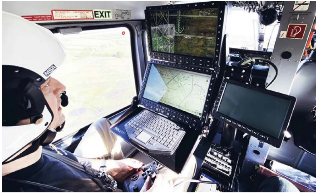
All set: a typical operator workstation for an aerial thermography installation. Advanced onboard processing speeds up fault location and identification tasks. Image: InfraTec
