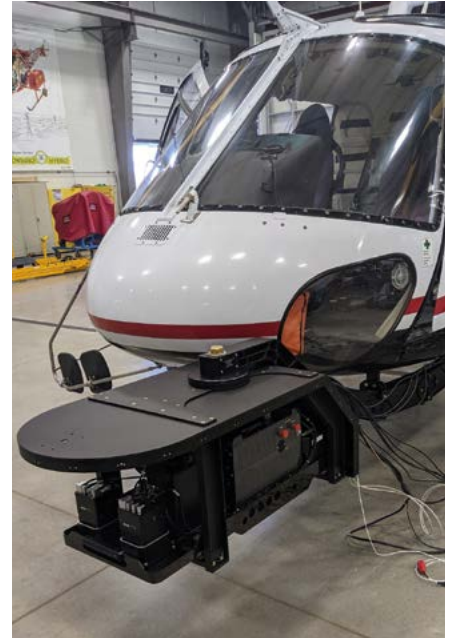
Payload: the Galaxy T2000 LiDaR and camera solution delivers ultra high resolution 3D measurements on electric infrastructure, as well as nadir and oblique imagery. The data is used for as-built infrastructure mapping, together with close-up inspection of assets. Image: Network Mapping Group/Teledyne Geospatial Technology
