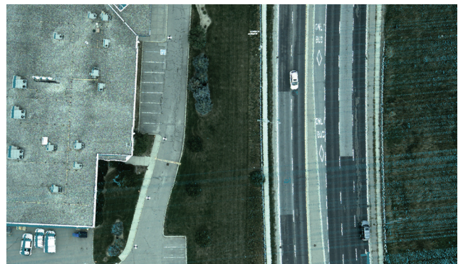
CLS-A colorized Lidar data from an engineering-grade survey of road and building hard surfaces.
