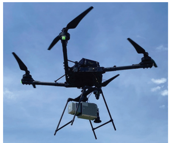
CLS-A Integrated with Freefly Alta-X UAV.
