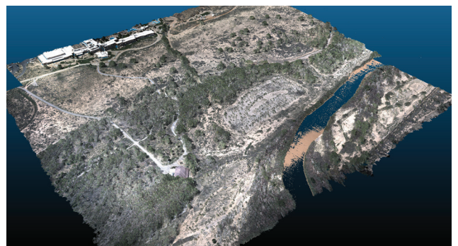
Colorized Topographic Survey collected with CLS-A.
