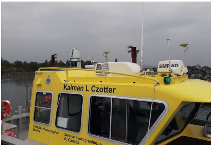
▲ Example installation of the Optech Polaris laser scanner on a coastal survey vessel. Image courtesy of the Canadian Hydrographic Service.
